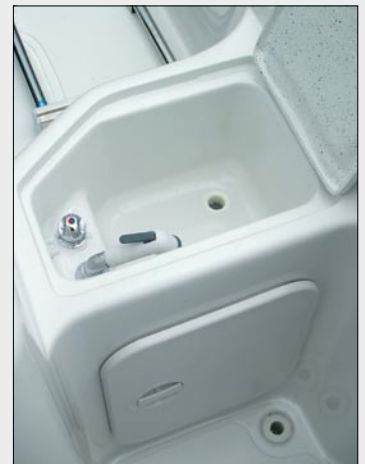
Cleanup sink and washdown hose
